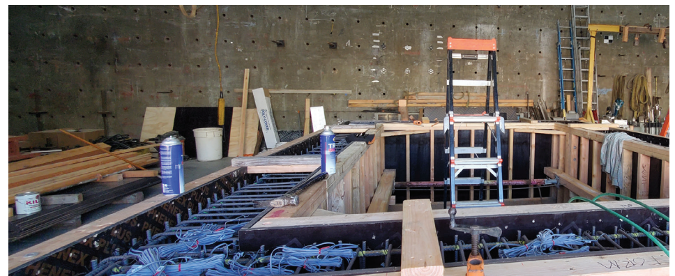
UCSD/California Department of Transportation (Caltrans) funded Project, where the researchers were casting a box tunnel to subject it to cyclic and fatigue loading.
