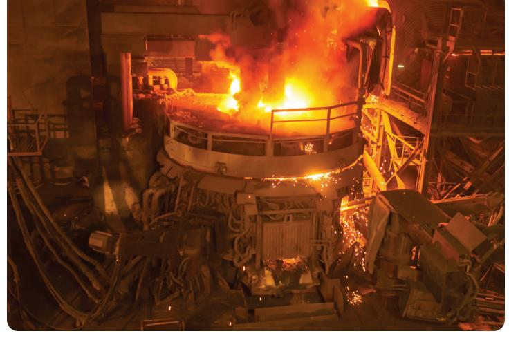
All steel reinforcing bar produced in the United States come from electric arc furnaces (EAF), as opposed to traditional blast furnaces, that greatly reduce CO2 emissions. Furthermore, steel mills are investing in new casting process that do not require reheating to create finished products.
