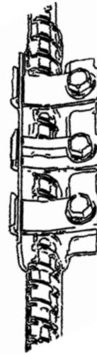
Figure 14 — Bolted strap coupling sleeve
