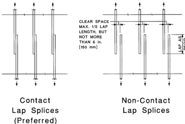
Figure 1 — Contact and non-contact tension lap splices
